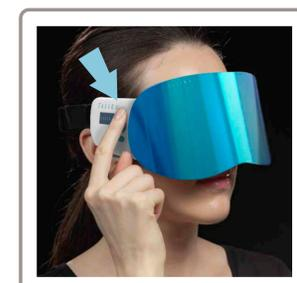
IF YOU FEEL ANY UNCOMFORTABLE ELECTRICAL SENSATION: you can either decrease the intensity by scrolling down or press START / SELECT / PAUSE to stop the device.
